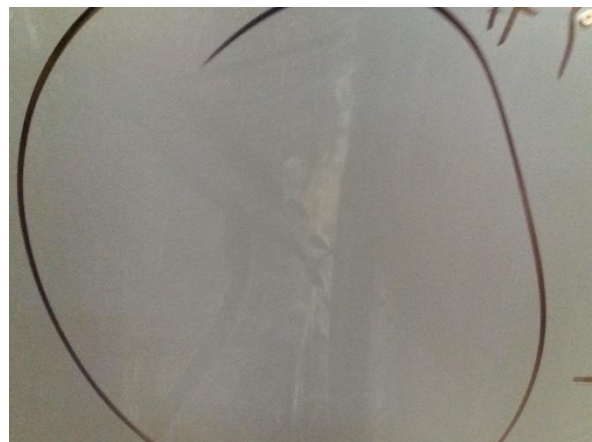
Plate 4.3: Soft body impact made no impression on the board.
